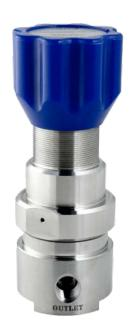
The MF-101 incorporates a large precision machined sensing element to control outlet pressures up to 35bar from a maximum 100bar inlet. The main valve is an unbalanced design to create positive shut off on gas or liquid applications against the PEEK seat.
