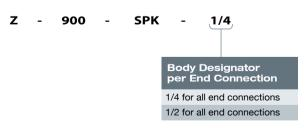
■ For oxygen applications work shall be carried out according to procedures for working with oxygen. In case spare kits are ordered for oxygen clean valves, such kits have to be ordered as oxygen clean by adding "-OC" designator. Example: Z-900-SK-1/4-VI-OC
