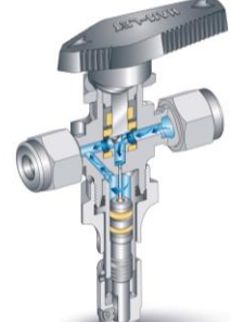
Full-Flow Mode Ball Valve's Handel is opened
