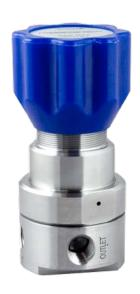
The BP-300 has been designed with a convoluted Inconel X750 diaphragm that lasts 50% longer than a typical stainless steel designs. Its compact simple design makes it ideal for general purpose applications, where accurate control of upstream pressure is required.
